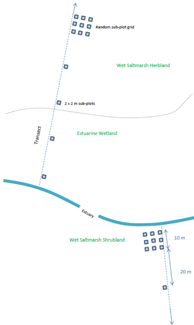
Figure 4. Example of grid and sub-plot transect layout for saltmarsh and related vegetation stratified by EVC (not to scale)
