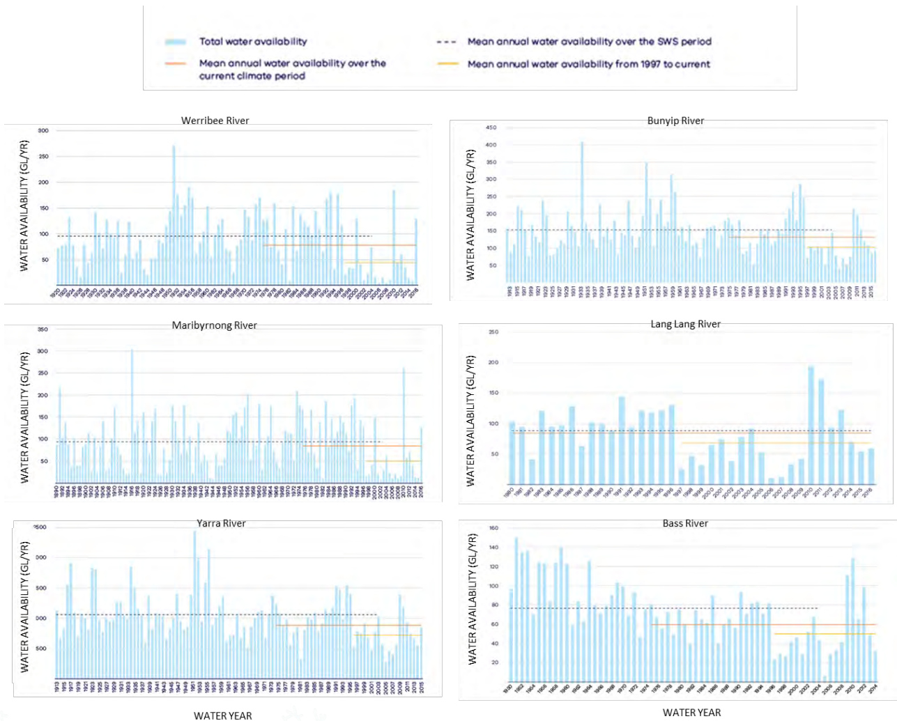
Figure 39. Annual water availability in six rivers of the Melbourne region (Government of Victoria 2020).
